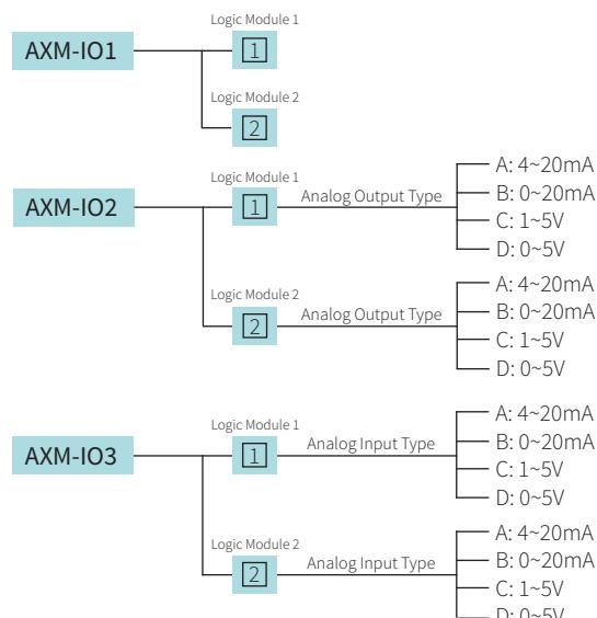
I/O Module Ordering Example: AXM-IO2-1A
